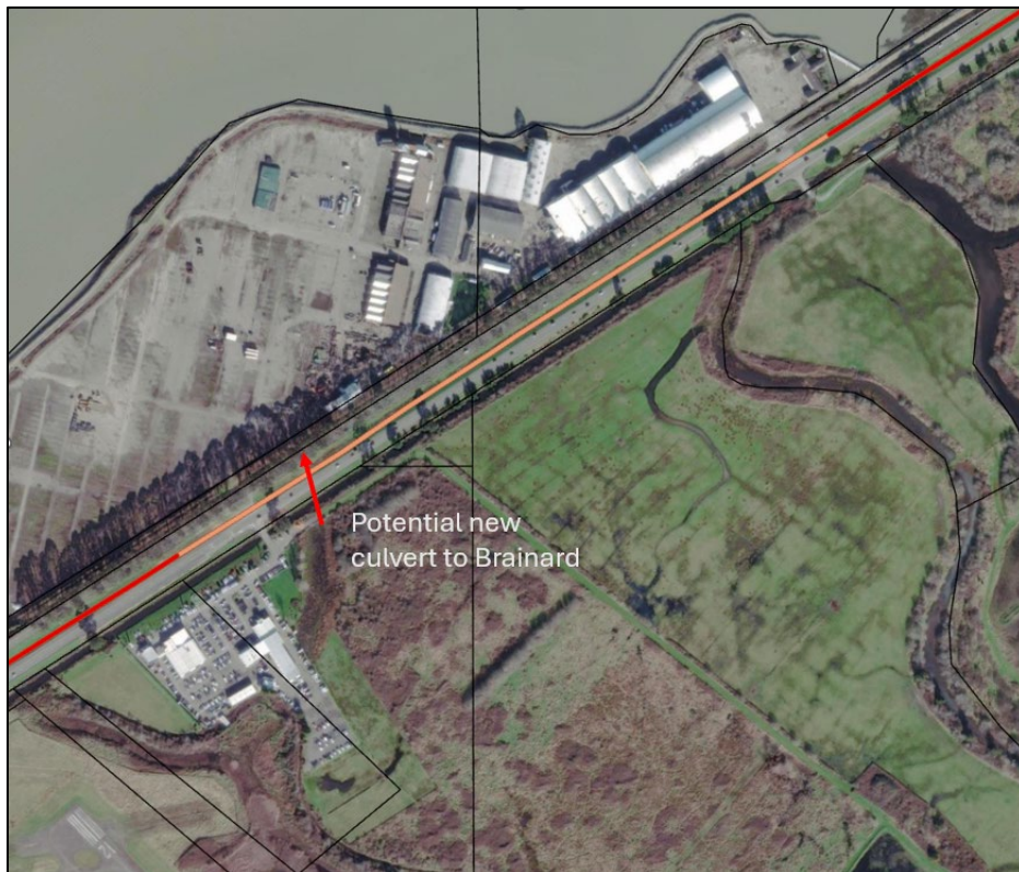
Figure 55. Map showing Segment 3 (orange line) which spans North Fay Slough to North Brainard. The adaptation options along this segment of the Corridor include a raised embankment with potential hydraulic connection to the old Brainard Mill site. Black lines outline individual parcels.
