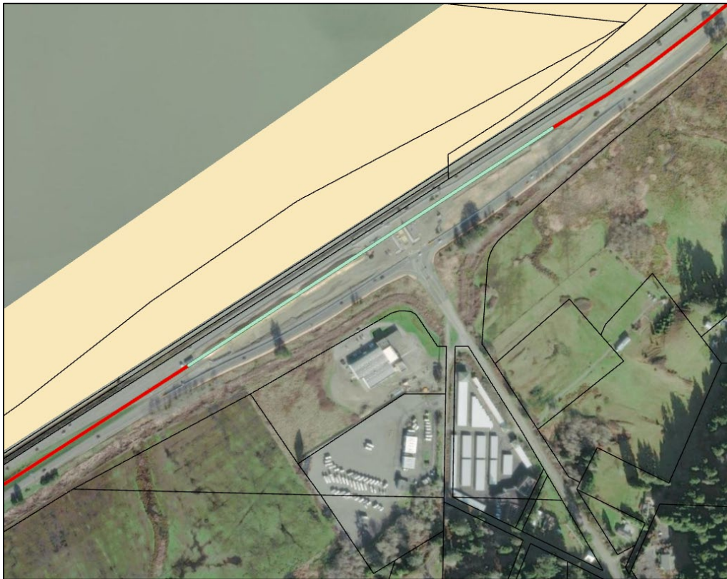
Figure 57. Map showing Segment 5 (green line) which spans South Indianola to North Indianola. No adaptation options are planned for this segment as elevations are greater than 16 ft NAVD88. The tan polygon indicates potential living shoreline location. Black lines outline individual parcels.
