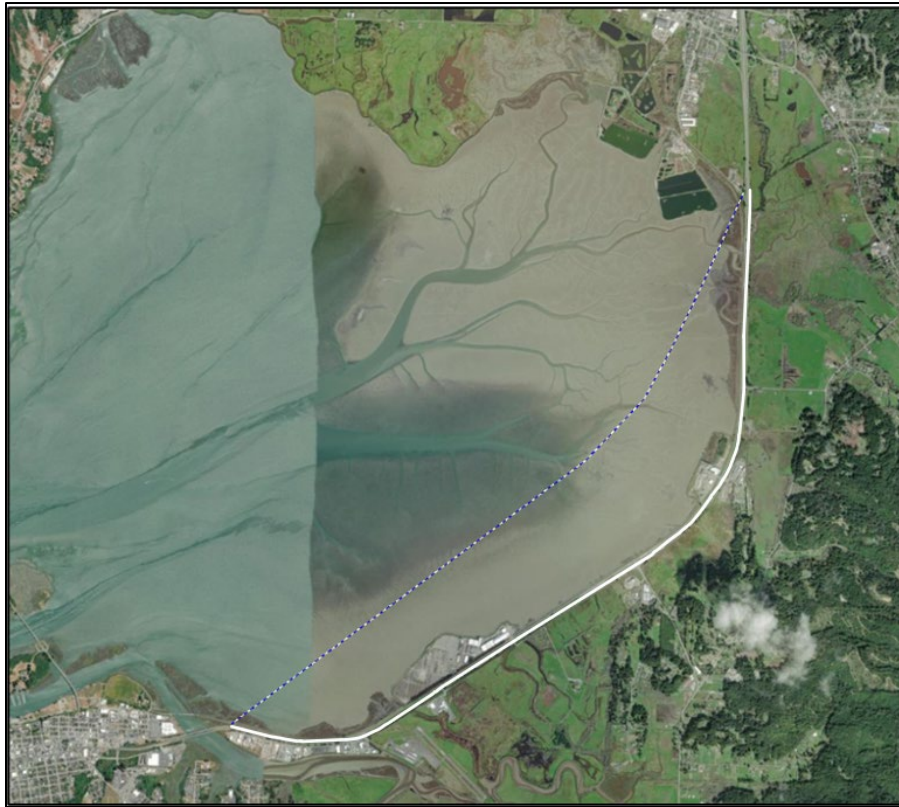
Figure 49. Example of full span viaducts across Arcata Bay (white and blue dashed line) and along current highway alignment (solid white line).
