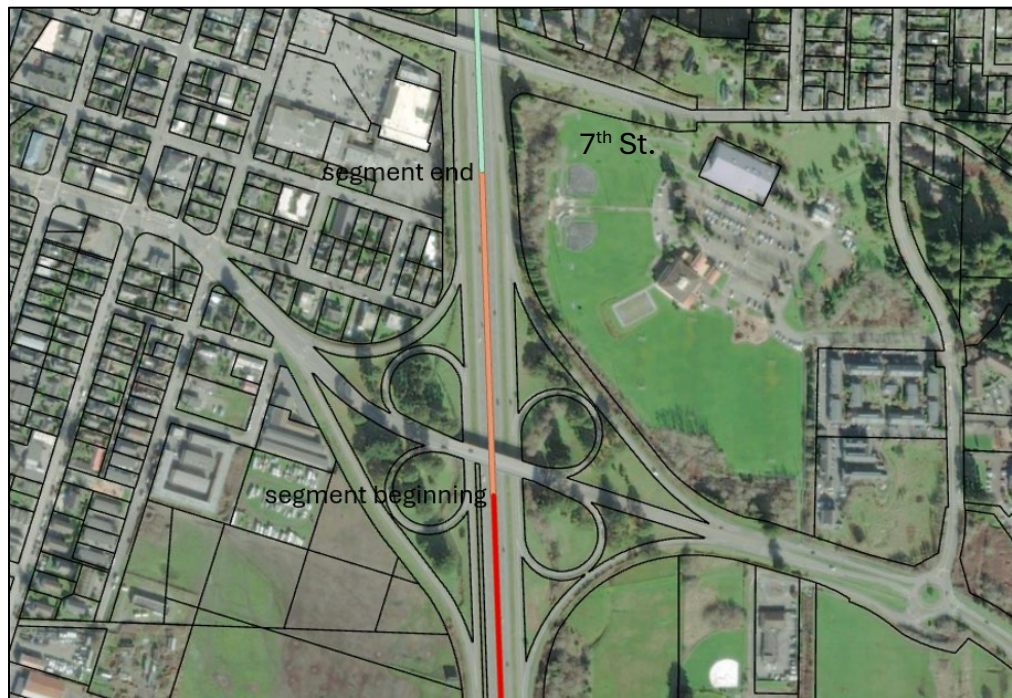
Figure 64. Map showing Segment 12 (orange line) which spans the SR 255/101 Separation Bridge to 7 th Street in Arcata. The adaptation options here include a raised embankment. Black lines outline individual parcels.
