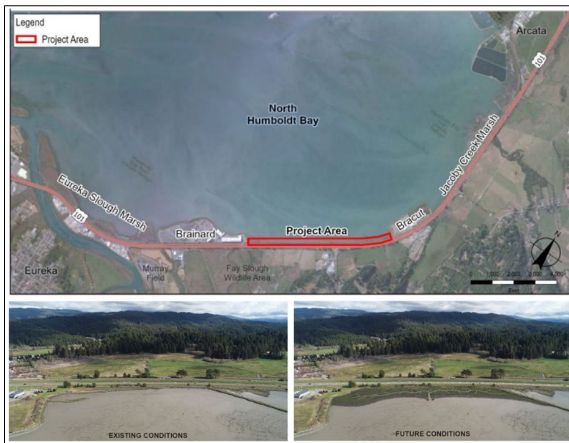
Figure 46. Living shoreline feasibility study. Top: Project area; Bottom: Existing conditions and visual simulation of living shoreline along the Corridor (from GHD, 2022).
