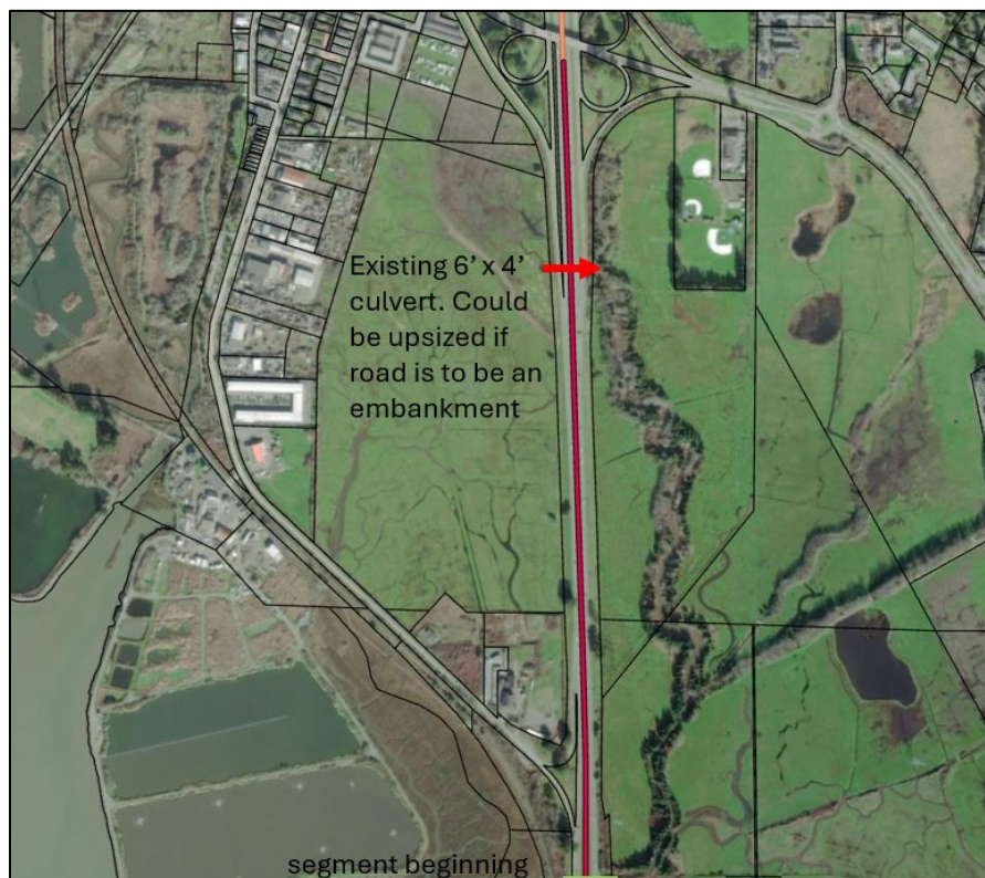
Figure 63. Map showing Segment 11 (red line) which spans South G Street to the SR 255/101 Separation Bridge. The adaptation options here include a raised embankment or viaduct with potential addition of a living shoreline (tan polygon) and upsized culvert. Black lines outline individual parcels.
