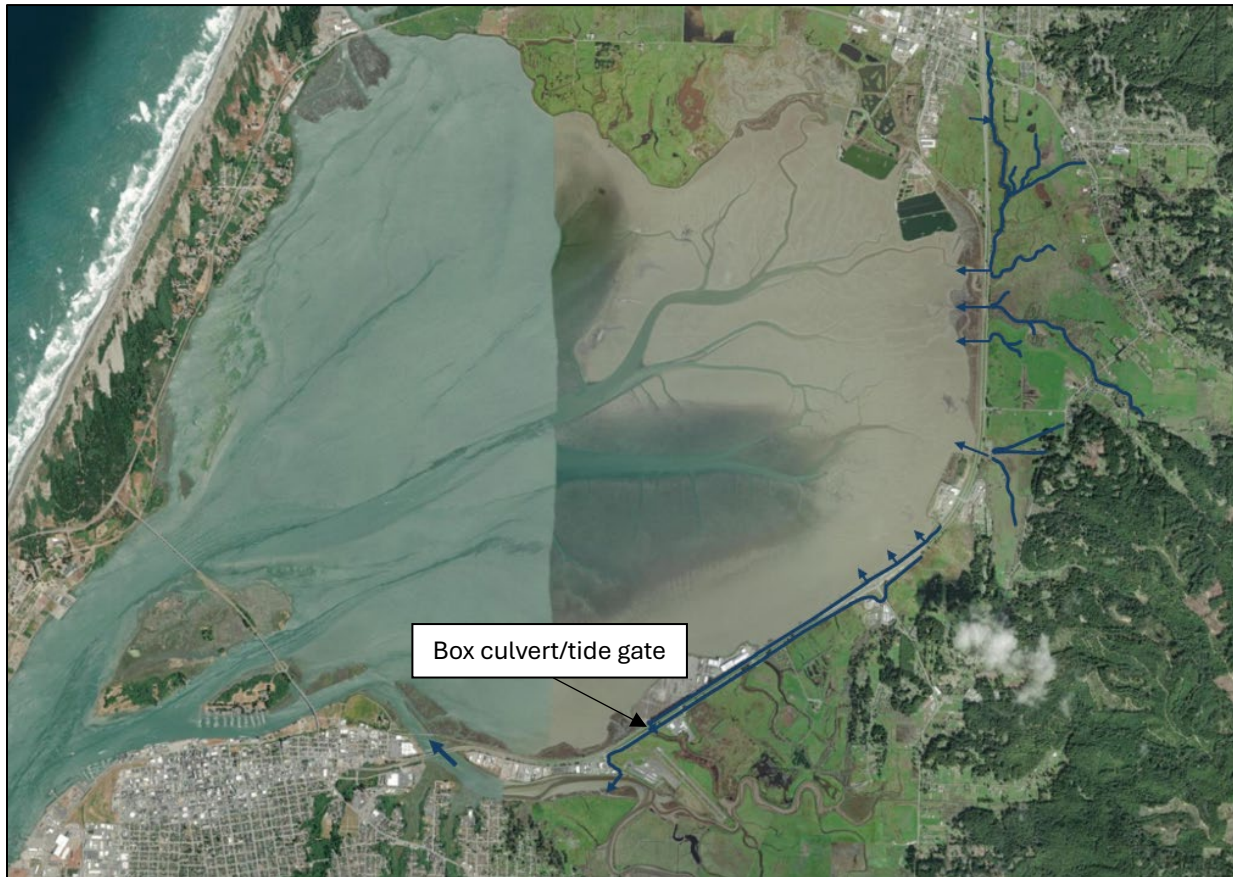
Figure 13. Simplified drainage pattern of water flowing out to the bay. Note that there is a box culvert and tide gate on the southern end of Brainard connecting drainage on the western side of the highway to the eastern side with an outlet to Eureka Slough.
