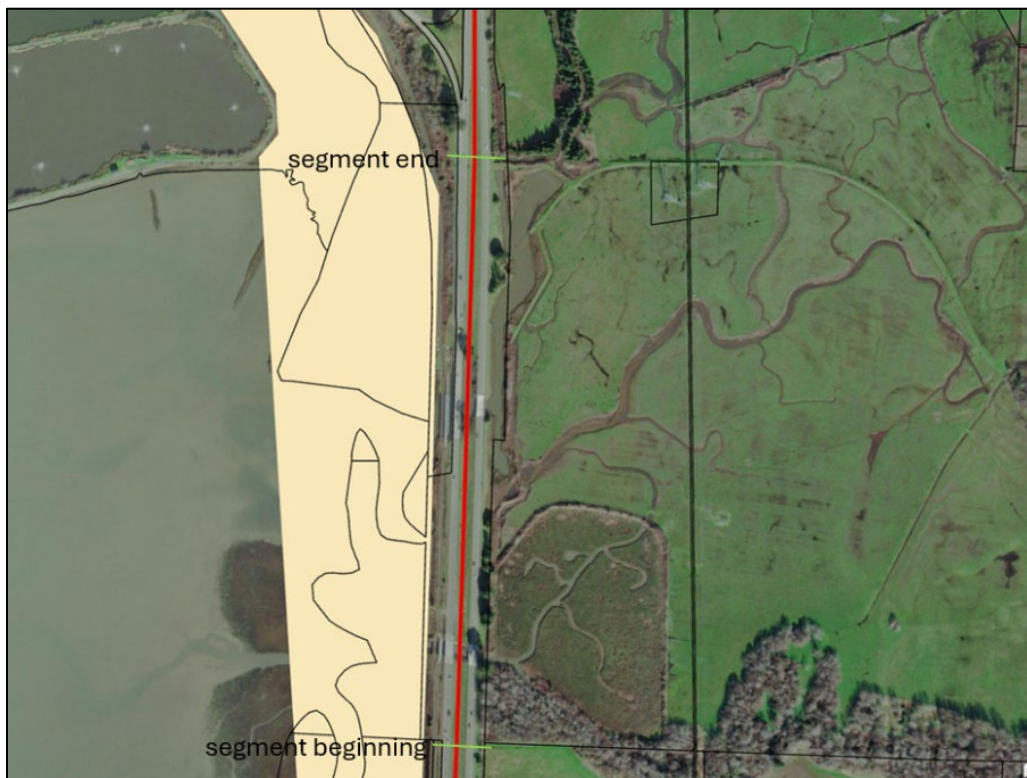
Figure 62. Map showing Segment 10 (red line) which spans Jacoby Creek Bridges to South G Street. The adaptation options here include a raised embankment or viaduct with potential addition of a living shoreline (tan polygon). Black lines outline individual parcels.
