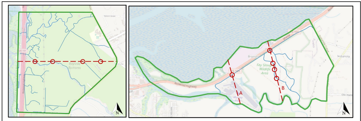
Figure 35. Model areas for the two local models developed for the CAIP hazard analysis. Left: Jacoby Creek/Bayside Bottoms model areas showing the cross section used to extract groundwater elevations for model comparisons. The red circles indicate locations where the cross section intersects blue line channels present in the City of Arcata stream channel GIS layer (City of Arcata 2024). Right: Fay Slough model area showing the cross section used to extract groundwater elevations for model comparisons. The red circles indicate locations where the cross section intersects blue line channels present in the USGS National Hydrography Dataset (USGS 2024). In both images the channel layer has been clipped to the model area.
