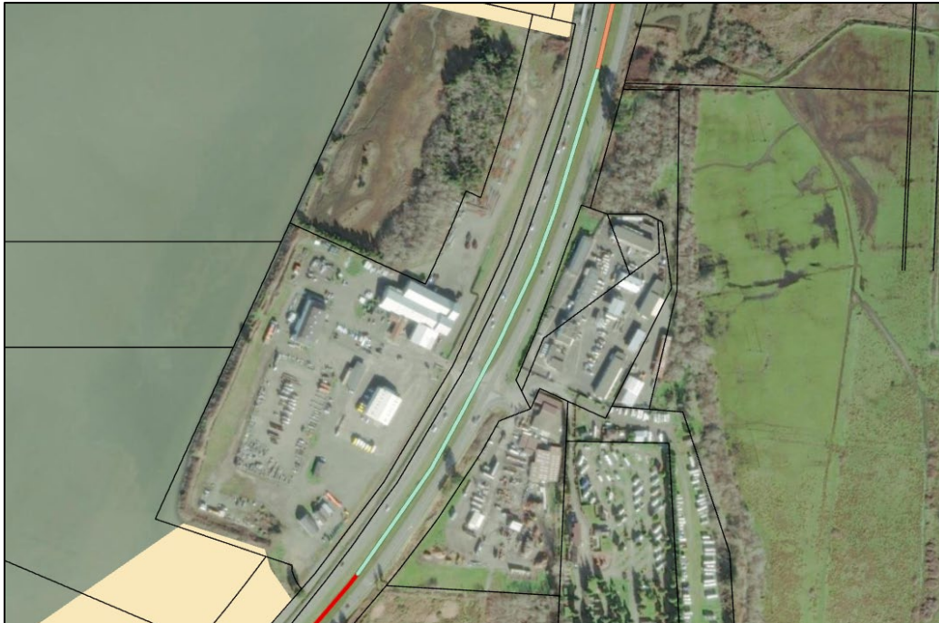
Figure 59. Map showing Segment 7 (green line) which spans South Bracut to North Bracut. No adaptation options are planned for this segment as elevations are greater than 16 ft NAVD88. The tan polygon indicates potential living shoreline location. Black lines outline individual parcels.
