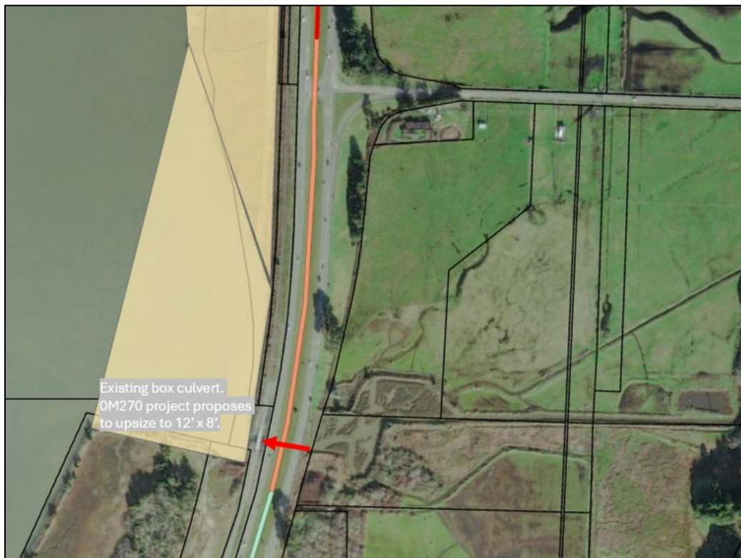
Figure 60. Map showing Segment 8 (orange line) which spans North Bracut to Bayside Cutoff. The adaptation option here includes a raised embankment with potential living shoreline and hydraulic connection to the bay. The tan polygon indicates potential living shoreline location. Black lines outline individual parcels.
