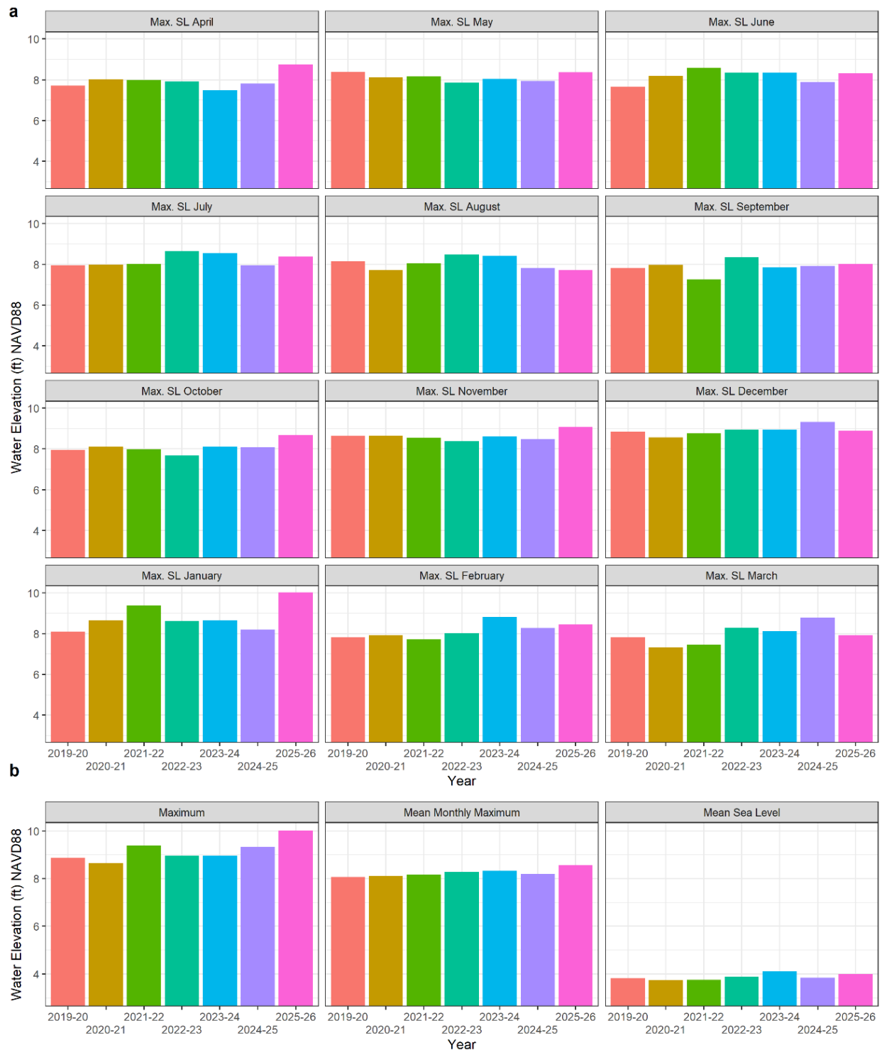
Figure 16. Maximum water elevation and summary statistics for the North Spit Tide Gauge for all annual reporting periods (April 1 through March 31), 2019 to 2026. a) Maximum water elevation (y-axis; ft NAVD88) by month (see individual plot titles) and year, b) From left to right: maximum, mean monthly maximum, and mean sea level (y-axis; ft NAVD88) summarized by year. Water elevation data from NOAA, 2026.
